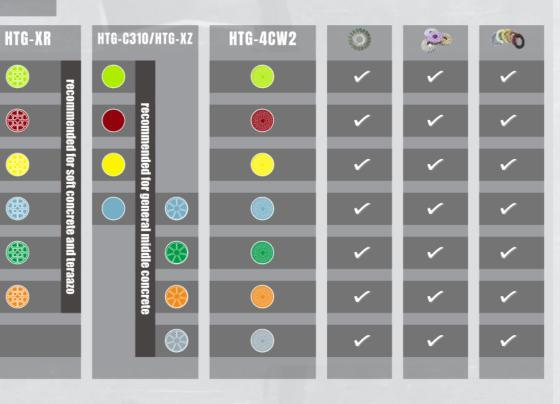
The mounting pad with the pre-installed patent designed resin discs is suitable for direct mounting on a trowel blade or other form of mounting plate in the market. Different polishing effects from cream to fine aggregate can be obtained by selecting the grit number of 1#-6#.
